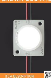
Crown DUO R13V12 modules are best for double sided light boxes. Equipped with elliptical lenses these modules are designed for depths ranging from 140 to 250 mm, can be installed with 60 – 200 mm step. Crown DUO R13V12 show extreme endurance at harsh working conditions (IP66) and have 3 year warranty with L70 for 25,000 hours.
